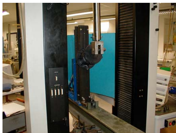
side pull applied to a support made up of a circular base, a circular head without tray with tabs and two sleeves
