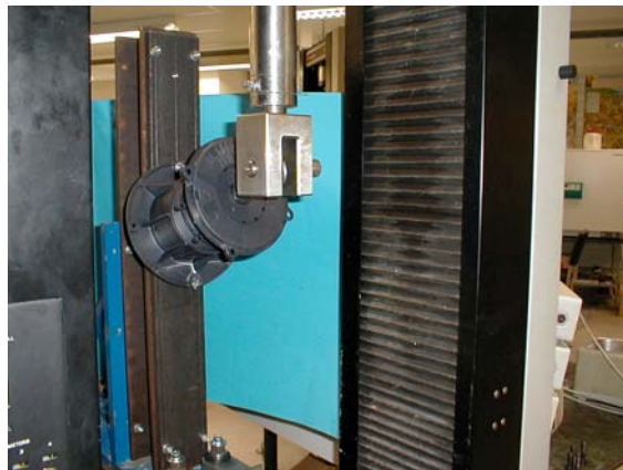
side pull applied to a support made up of a circular base and a circular head without tray with tabs
