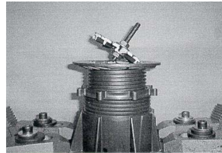
Photo No. 5 The web remains attached to the head of the BUZON DPH5 pedestal
